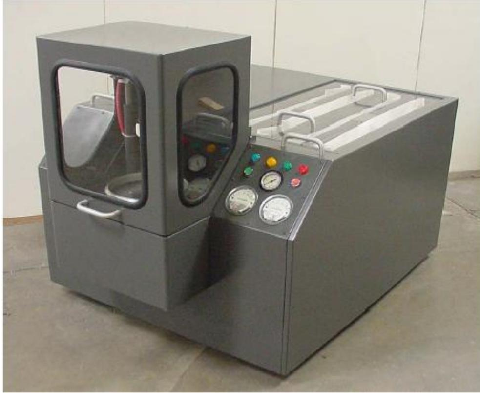
Figure (76): diesel particulate filter cleaning unit, ( source: [www.meca.com](http://www.meca.com)).
